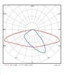
TYPE I The Type llens has beam angle of 70\*140 degrees. In the IESNA Standard, The Type distribution is great for lighting walkways, paths and sidewalks. It is generally applicable to where the mounting height is approximately equal to the roadway width.
